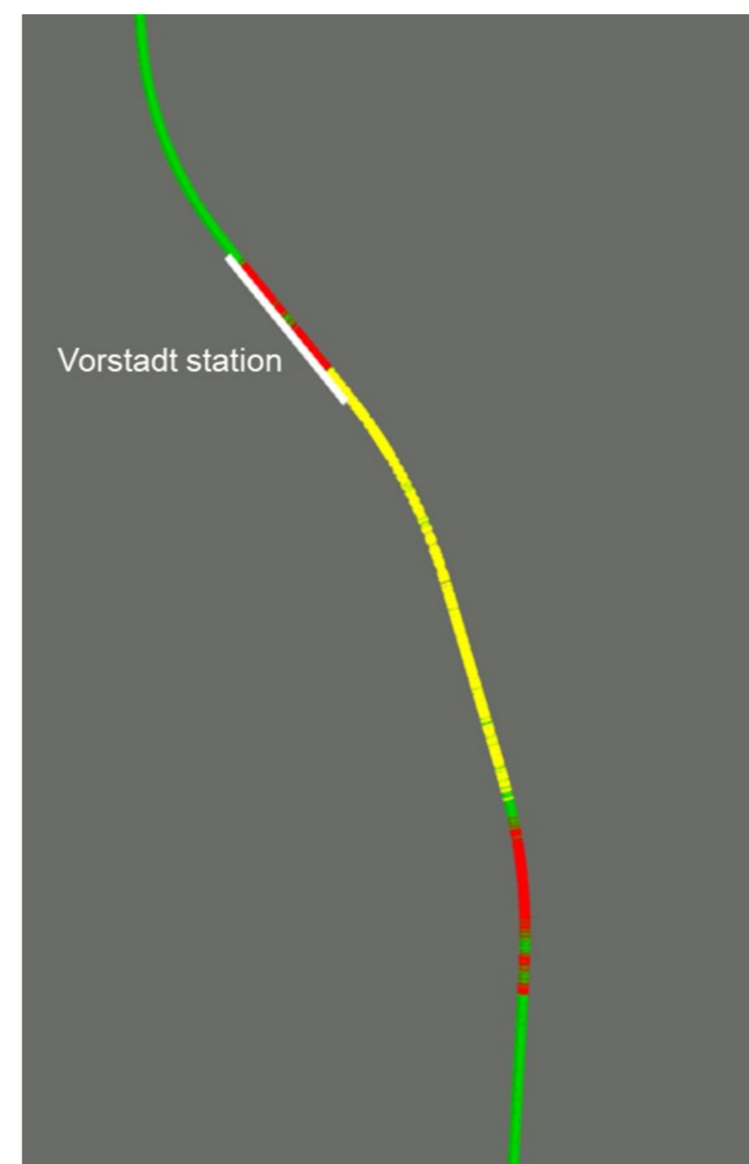
Visualization of longitudinal acceleration measured from the car body.
